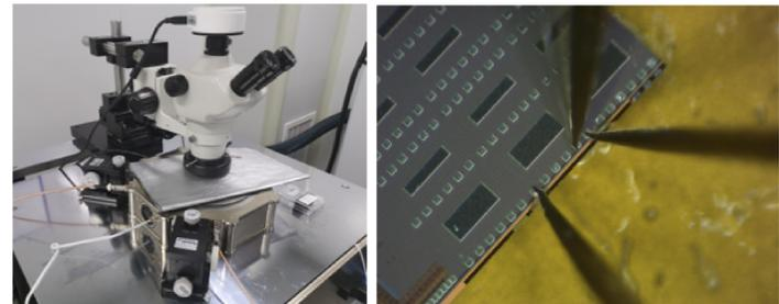
The IV and CV test probe station.
