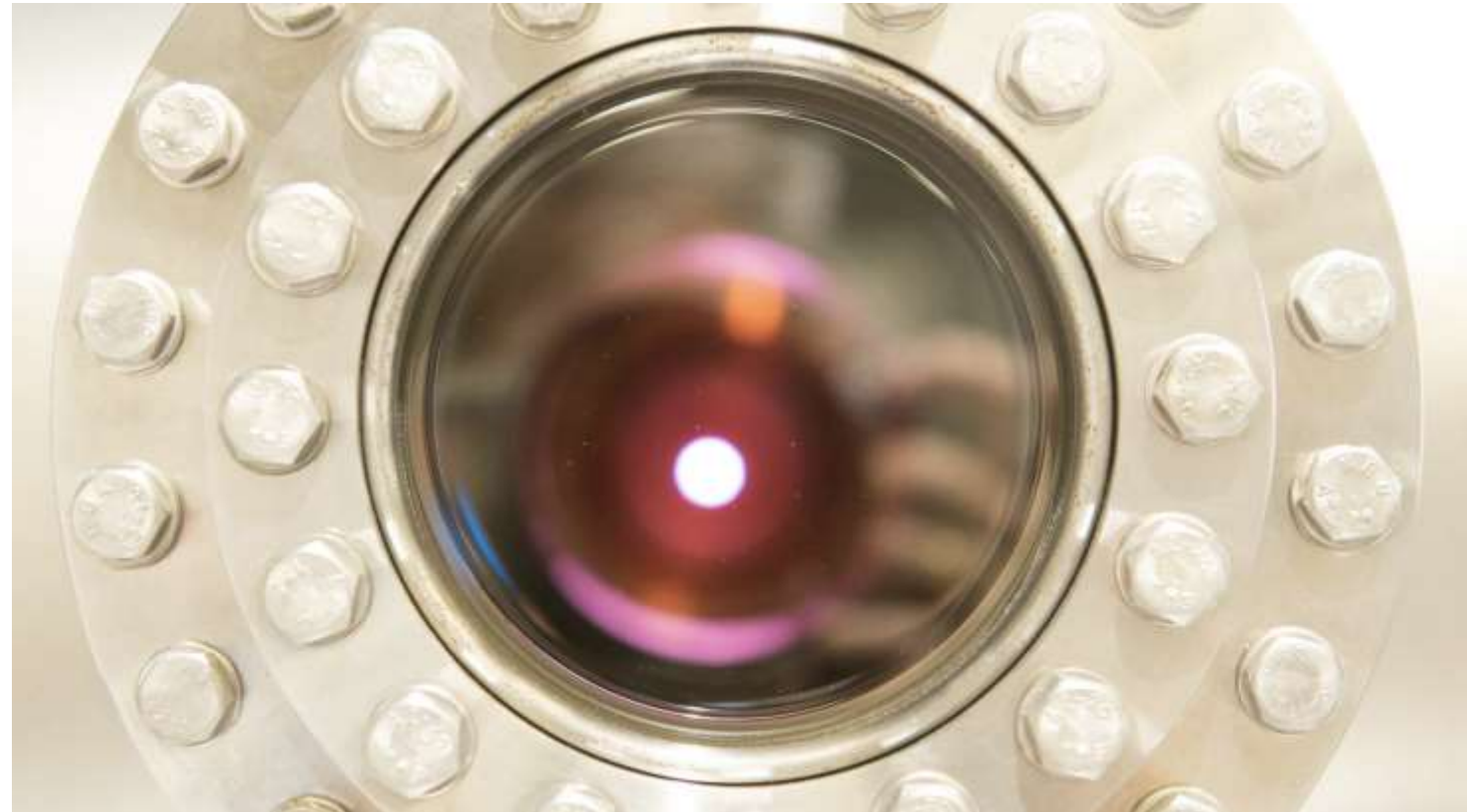
View of white, glowing ball of proton plasma in the Ion Source.
