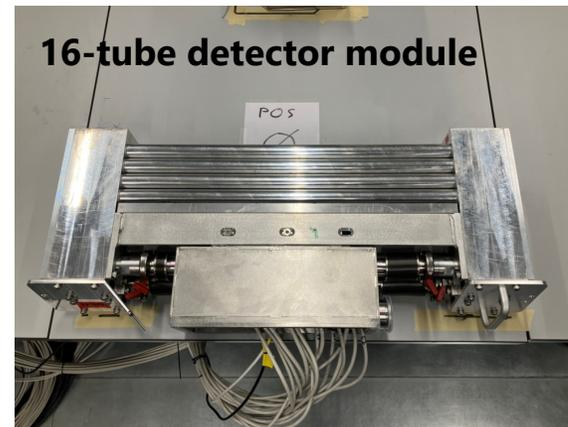
Multi-tubes coated with  $\sim 1 \mu\text{m}$  of  $^{10}\text{B}_4\text{C}$
