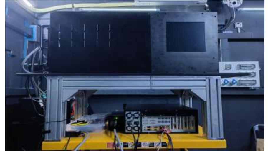
The maximum FOV is 220mm\*210mm, and the best spatial resolution is 25 μm measured at ENRI
