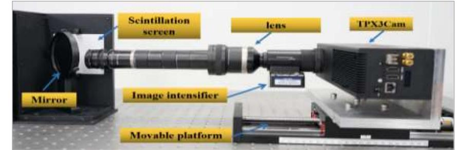
Energy resolution neutron imaging detectors can achieve high time resolution and high spatial resolution at the same time.
