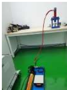
Clamp cell loading system
