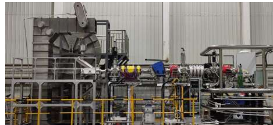
Low energy high current ion beam coupled with granular flow target thermal measurement platform
