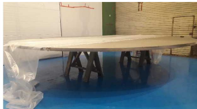
Bottom plate welding completed
