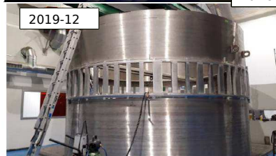
Lower body with rear window tack welded
