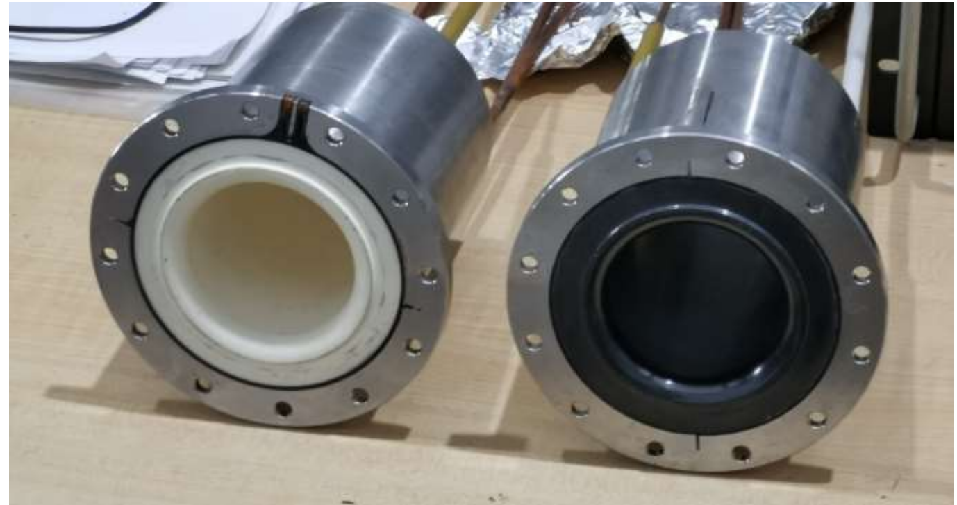
\text{Al}_2\text{O}_3 (left) and \text{Si}_3\text{N}_4 (right) plasma chambers for thermal and mechanical test
