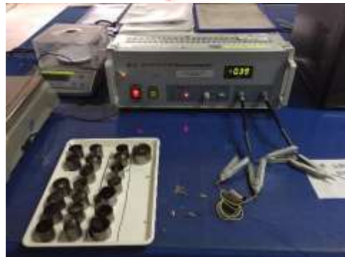
Testing the impact of the coating to the performance of small MA cores.
