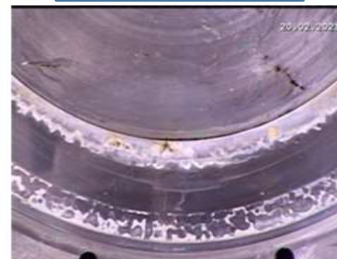
Seal surface at Helium vessel end by camera observation
