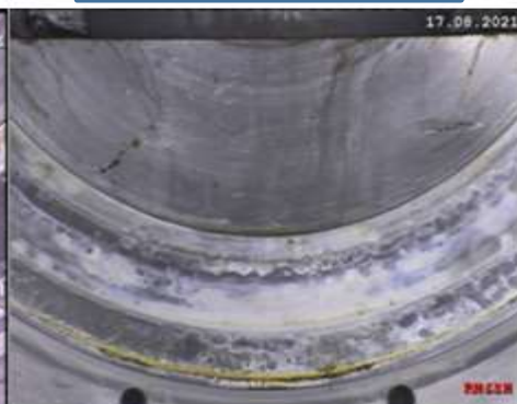
Seal surface at Helium vessel end by camera observation
