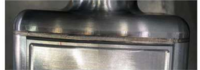
vacuum vessel electron beam welding for DPHM
