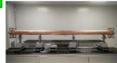
S-band Accelerating structure
