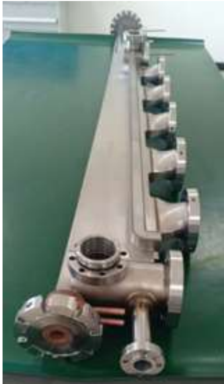
Stainless steel chamber with pumps, photon absorbers and end mask, and copper is coated inside.
