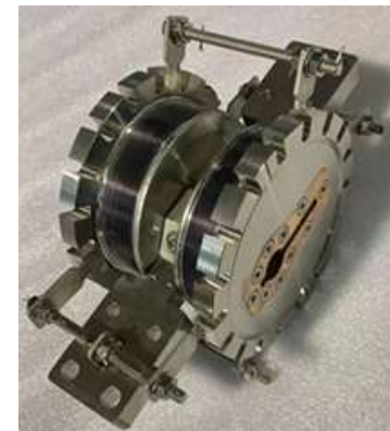
RF shielding bellows with double-fingers type, and BPM module is integrated.
