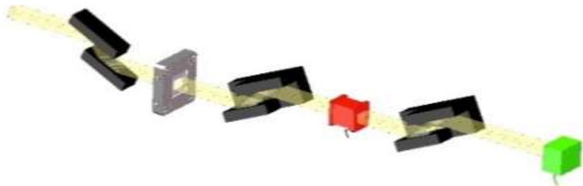
Rocking curve measurement layout
