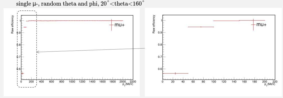
Raw efficiency: tracking efficiency before kalman fitting
