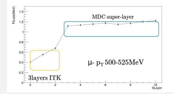
$\mathbf{p}_{\mathrm{T}}$  reduction(vs initial value) when the particle enters the detector
