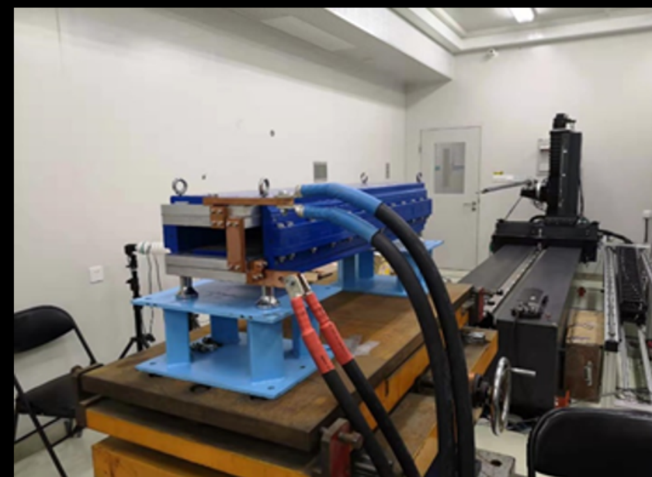
iron-core dipole magnet
