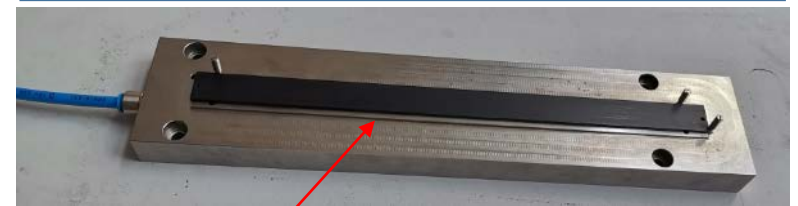
Vacuum plate for flex and CFRP support fixation
