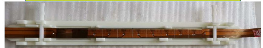
Vacuum plate for flex and CFRP support fixation
