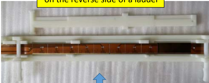
Tooling for mounting module on the reverse side of a ladder
