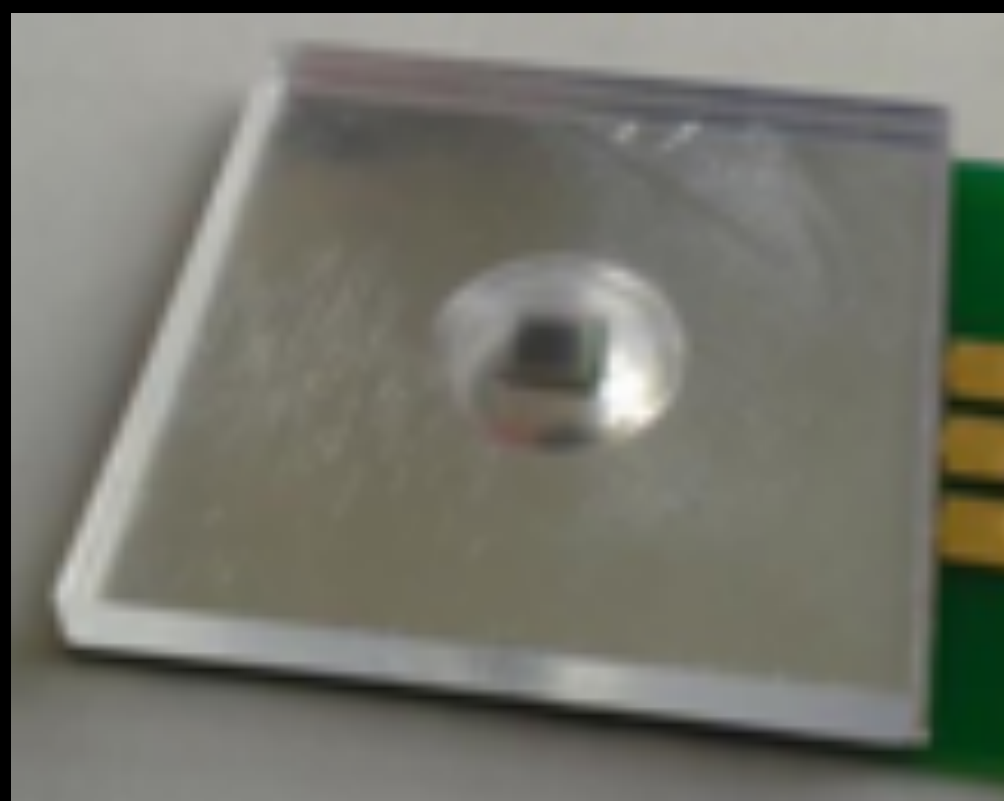
Embedded SiPM into Scintillator
