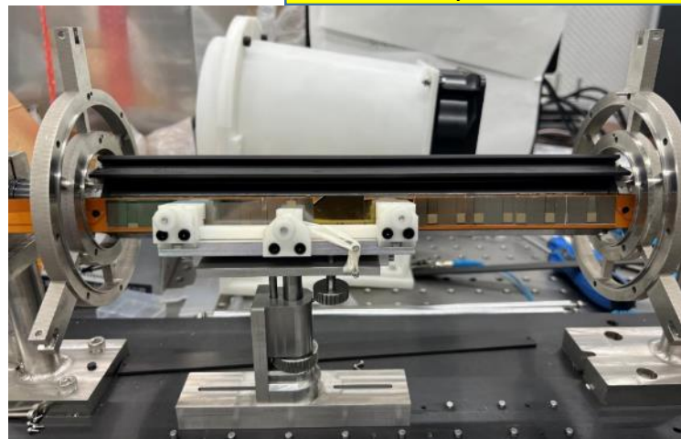
Formal parts - ladder loading test
