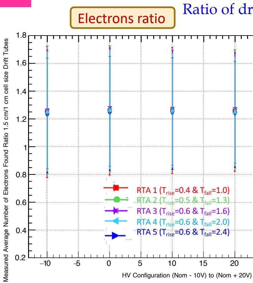
Ratio of drift tube size (1.2/0.8)
