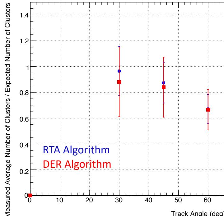
➤ Undercounting at  $\alpha > 45^\circ$  due to high electron peaks density.
