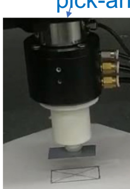
Placing dummy sensor
