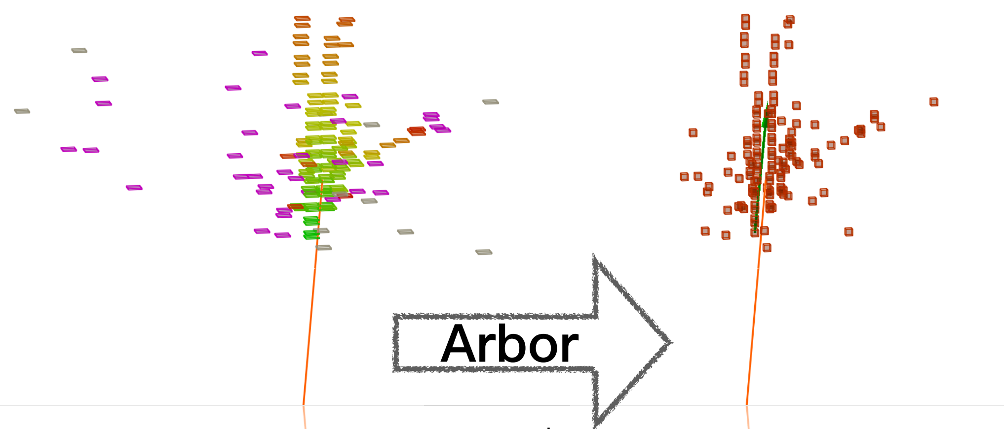
Event display of a 10 GeV \pi^\pm shower in ECAL, (left) without clustering and (right) after clustering by Arbor. The color of the hits in the left figure represents the true time.
