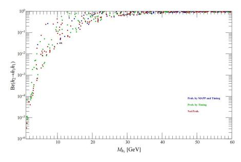
Green points are probed by CMS-Timing, but not by MAPP. CMS-Timing can probe **a lot more** 1st-order EWPT points. There are still appreciable points not probed by any of LLP detectors.
