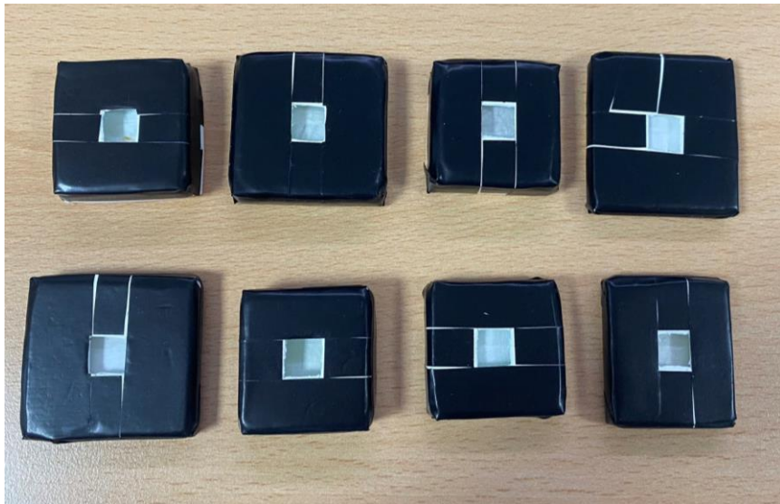
Glass tiles wrapped with Teflon and black tapes
