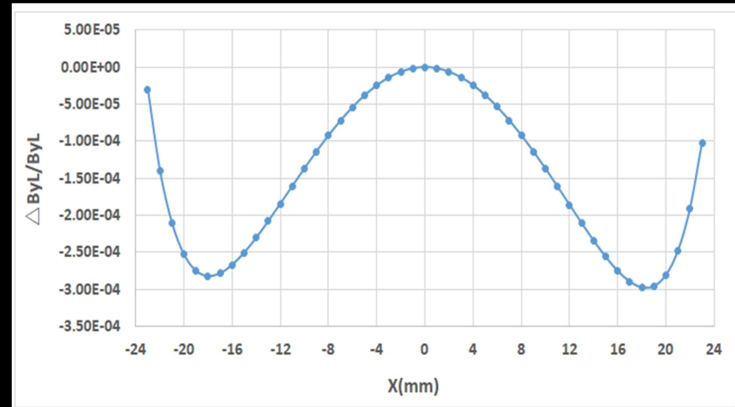
**Permanent magnets added at the end to help keep the beam uniformity within the MOST2 requirements**
