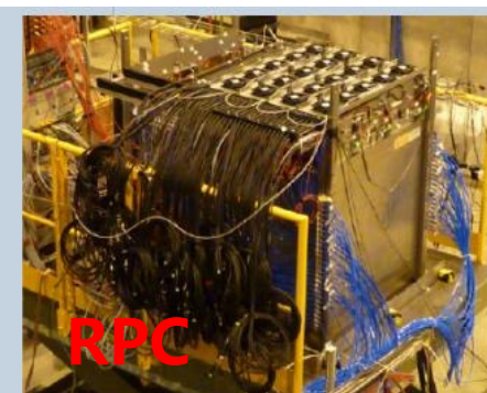
GRPC-SDHCAL, Fe: 48 layers, 1 \times 1 \text{ cm}^2 cells
