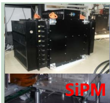
Sc-W ECAL: 30 layers, 1 \times 4.5 \text{ cm}^2 cells
