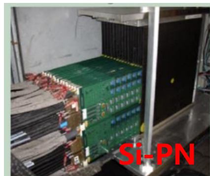
Si-W ECAL: 30 layers, 1 \times 1 \text{ cm}^2 cells
