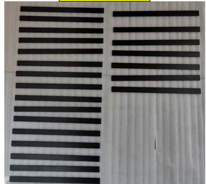
For the prototype, the CFRP laminate is slightly thicker than the previous fabrication test. Due to COVID pandemic, a new company that can make it before beam test was chosen to make the ladder support.
