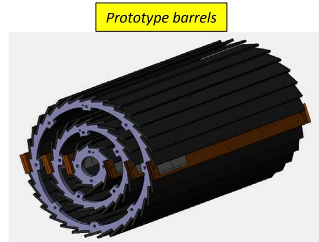
*For prototype beam test: 6 ladders are mounted on one line, others are bare CFRP ladder support.*
