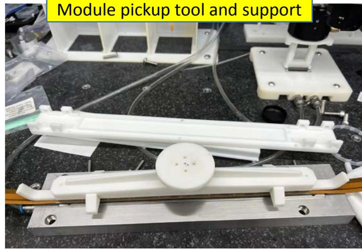
Vacuum chuck for sensors array
