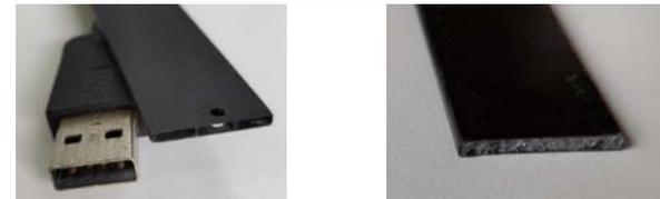
Aiming to reduce material, the CFRP laminate has to be very thin and the fabrication is very challenging.
