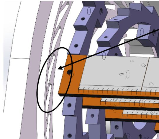
The convex ring provide a transition region for flex routing.
