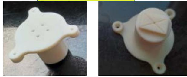
Vacuum plate for flex and CFRP support fixation
