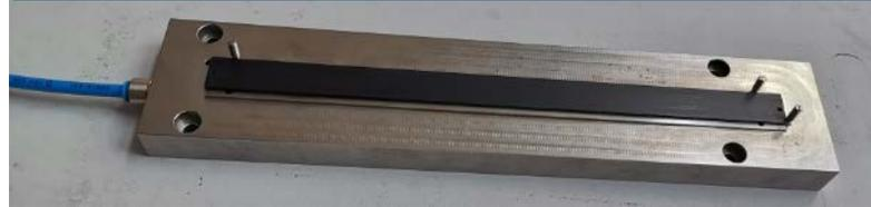
Module pickup tool and support
