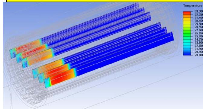
Chip temperature under cooling during beam test:
