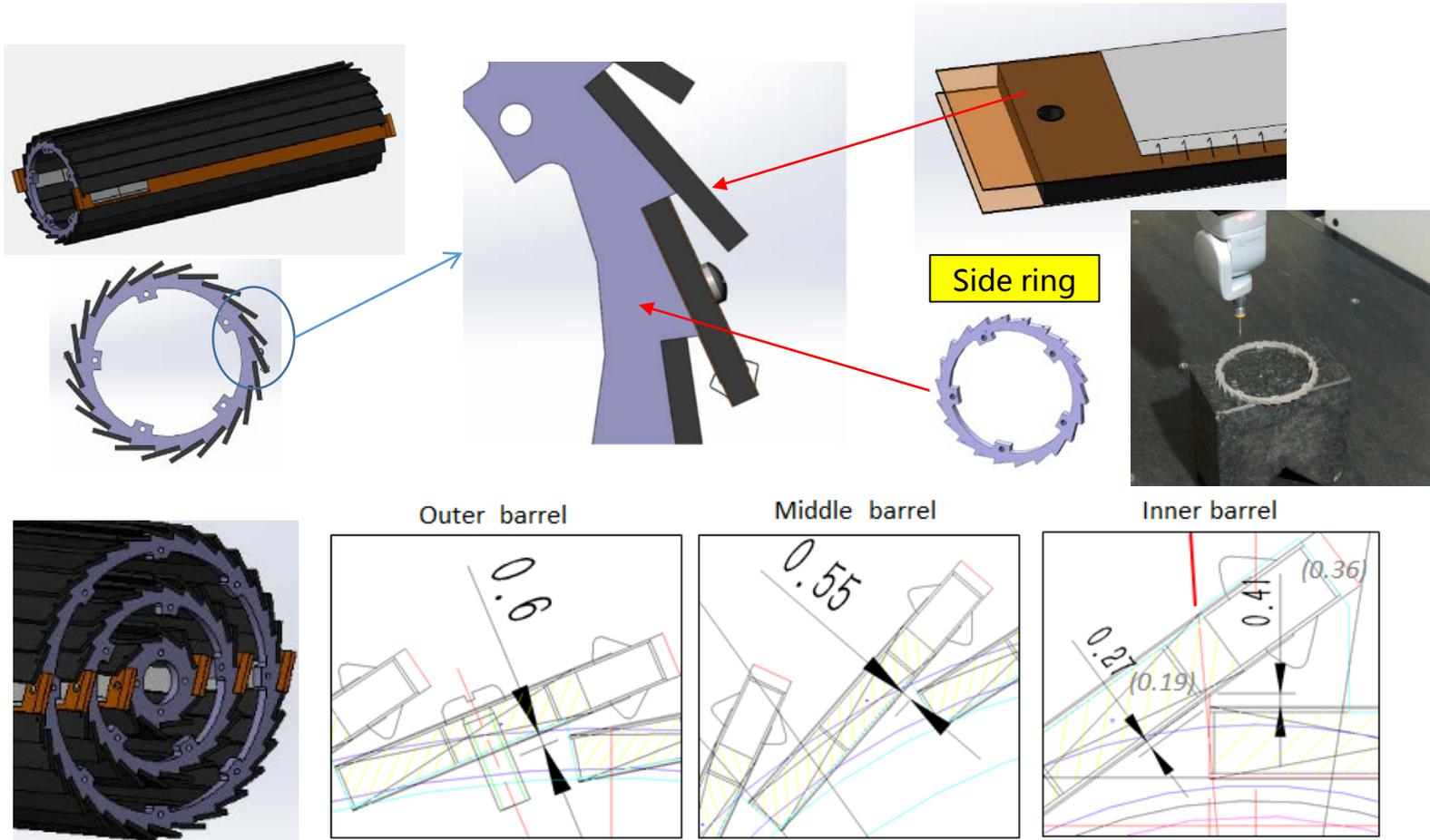
Very high precision is required for the CFRP support and barrel support.
