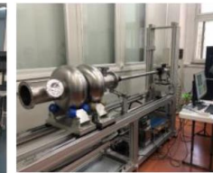
Cavity inspection camera and grinder
