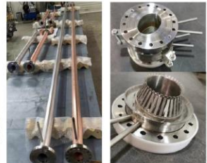
Vacuum pipes and RF shielding bellows
