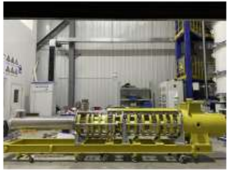
Klystron No. 2 Efficiency 77% (2021)
