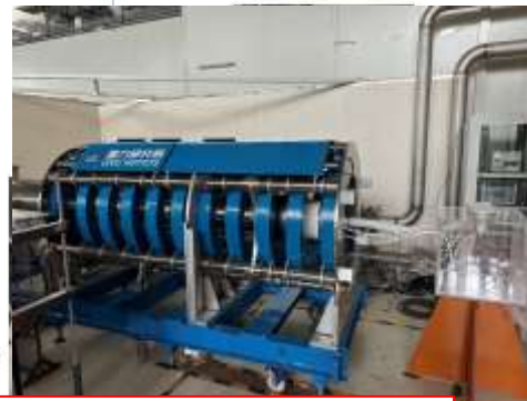
Klystron No. 3 (MB) Efficiency 80.5% (under fabrication)
