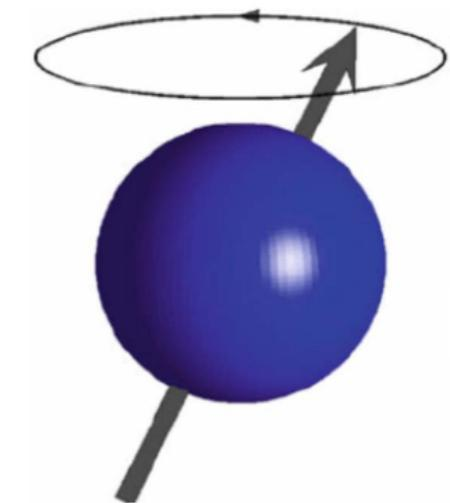
$$\boldsymbol{\Omega}_{\text{MDM}} = \boxed{\frac{g\mu_B}{\hbar}} \left( \mathbf{B} - \frac{\gamma}{\gamma+1} (\boldsymbol{\beta} \cdot \mathbf{B}) \boldsymbol{\beta} - \boldsymbol{\beta} \times \mathbf{E} \right)$$
