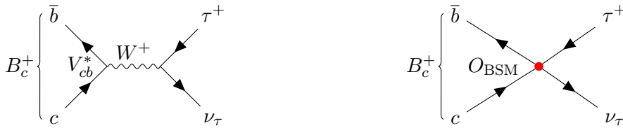
Figure 11: Illustrative Feynman diagrams for the decay B_c^+ \rightarrow \tau^+ \nu_\tau . LEFT: SM example. RIGHT: BSM example.
