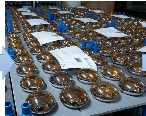
Potting and Leakage test @HZC
