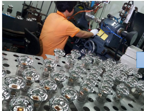
Production and test of bare PMT @HZC
