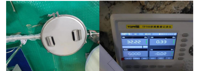
Leakage test after installation
