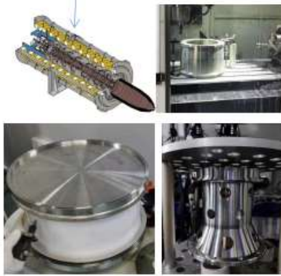
Klystron No. 3 (MB) Efficiency 80.5% (under fabrication)
