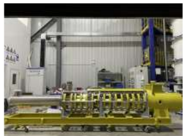
Klystron No. 2 Efficiency 77% (2021)
