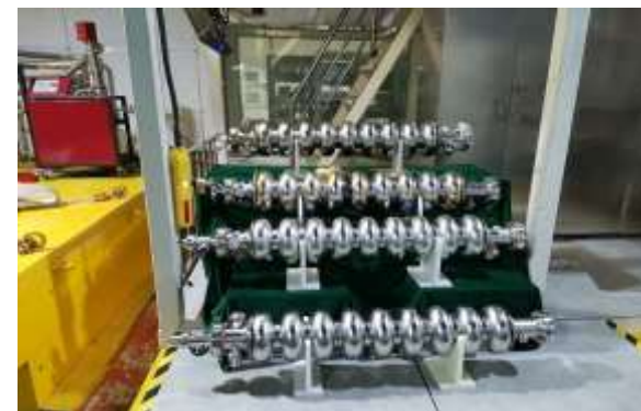
1.3 GHz High Q Mid-T Cavity Horizontal Test
