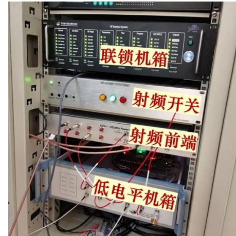
Digital LLRF system Stable operation since 2019
