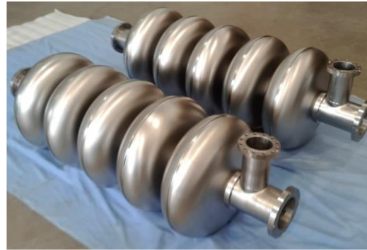
650 MHz 5-cell cavity (beta 0.82)
