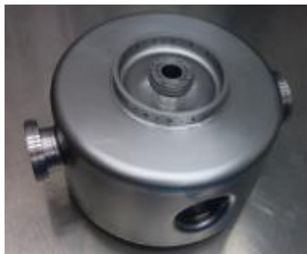
325 MHz Spoke cavity (beta 0.21)
