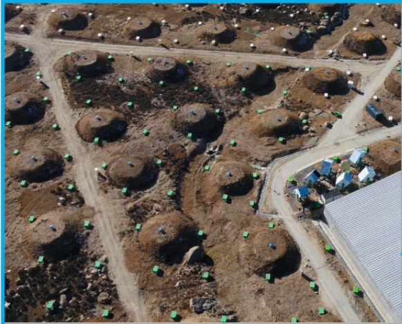
KM2A: (1.3 km 2 ) Electromagnetic Particle Detectors (ED) Muon Detectors (MD)
