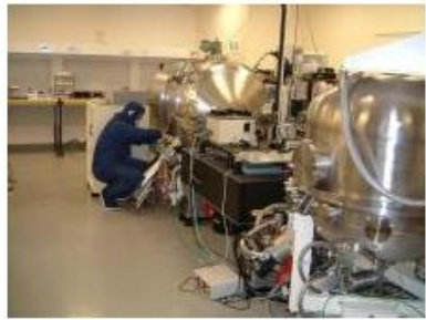
1m diameter chambers in clean assembly area
