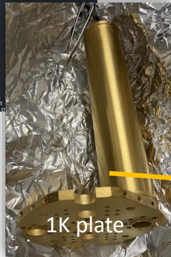
The "1K plate" (right) manufactured in workshop, prepared and installed into a Scanning Tunneling Microscope (STM) in Oxford Physics
