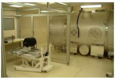
2.2m Chamber with vibration isolated optical bench
