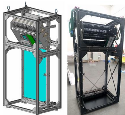
First test-beam with half-length quartz model in proto-TORCH with 2 MCPs
