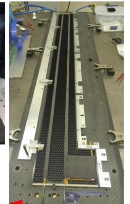
Bus Tape(left) and core assembly (right) Bus Tapes designed in EEG Manufactures in Photo fabrication
