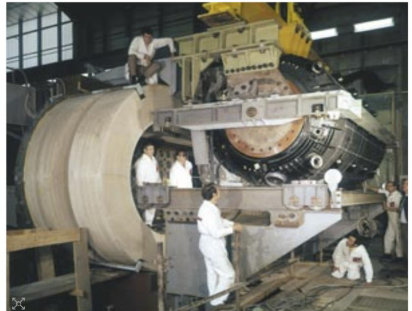
Fig. 1. The Gargamelle heavy-liquid bubble chamber, installed into the magnet coils, at CERN in 1970.
