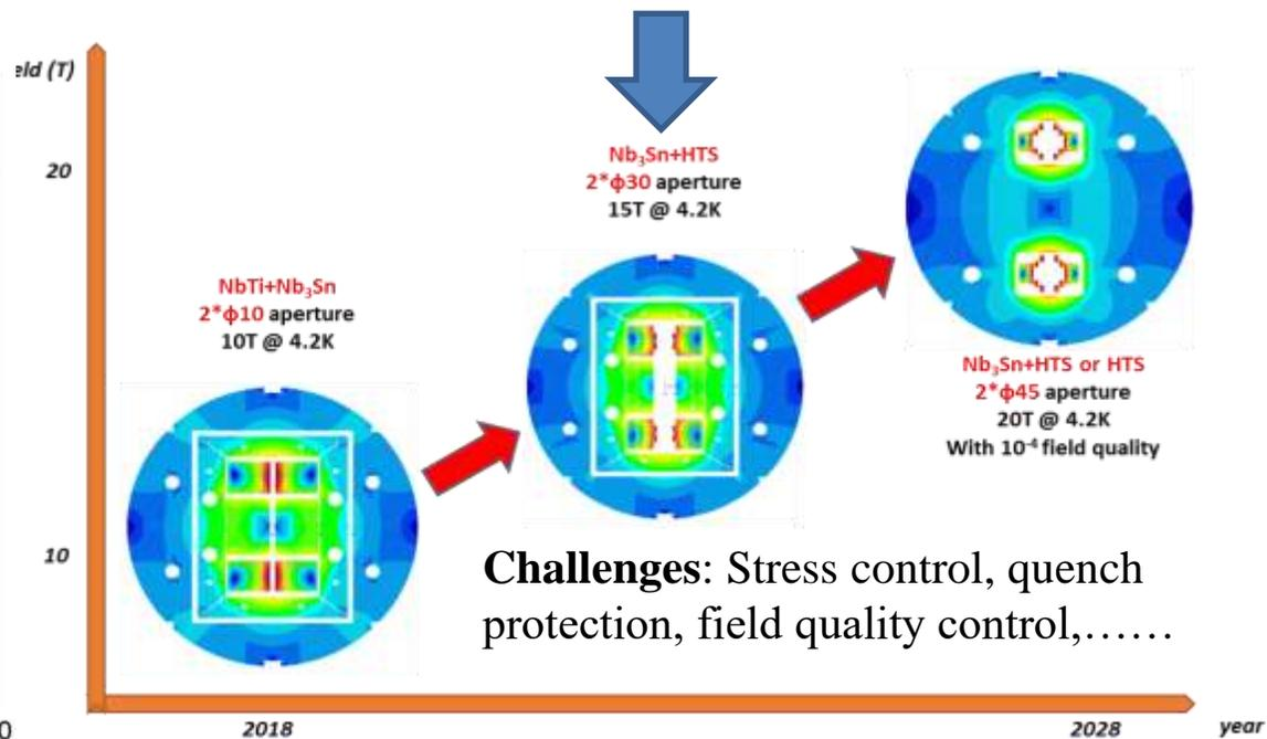
Dual aperture superconducting dipole achieves 12.47 T at 4.2 K
