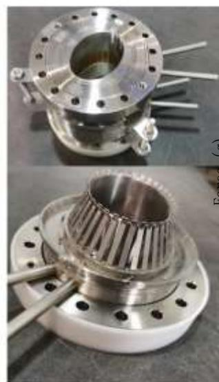
Vacuum pipes and RF shielding bellows
