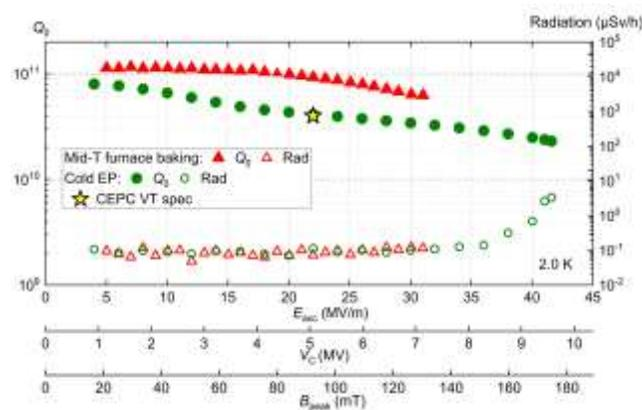
High G High Q 650 MHz 1-cell Cavity
