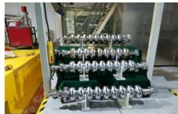
Mid-T (medium temperature furnace baked) cavities have higher gradient and Q than Nitrogen doped cavities with **less EP process (1 vs 3)**
