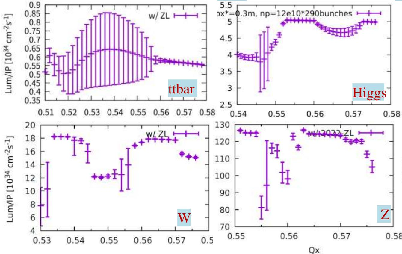
Beam-beam simulation results are **consistent** with the TDR parameter tables.
