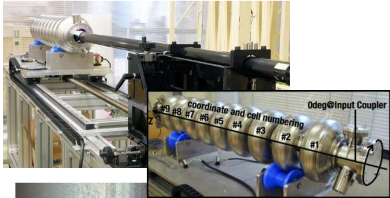
Cavity inspection by Kyoto camera
