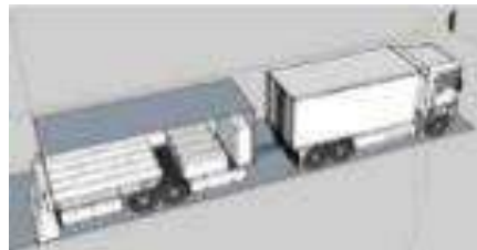
Electron beam onto asphalt to harden it and extend its life.
