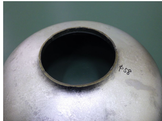
Successfully formed iris after improving the fabrication process
