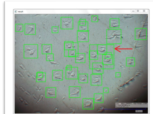
Figure 1: This is the output image for one of the positive test pictures from the Easy folder. One of the false positives is indicated by the arrow. It counted as a false positive for two reasons: more than 50% of contained defect area was contained in other, true positives, and it contained defects separated by more than 10 \mu\text{m} .
