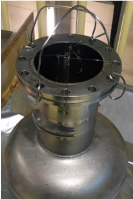
1st cavity coating
