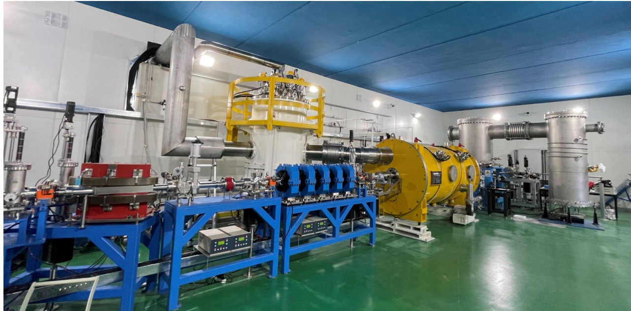
650 MHz test cryomodule with 2x2-cell cavities. Beam test soon.
