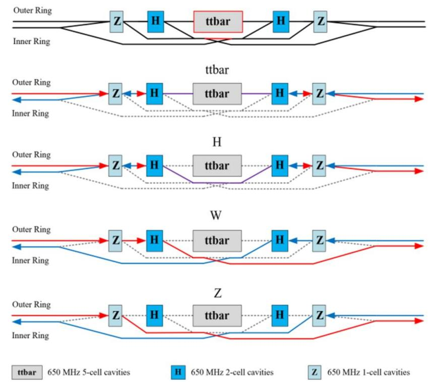
ttbar 650 MHz 5-cell cavities    H 650 MHz 2-cell cavities    Z 650 MHz 1-cell cavities
