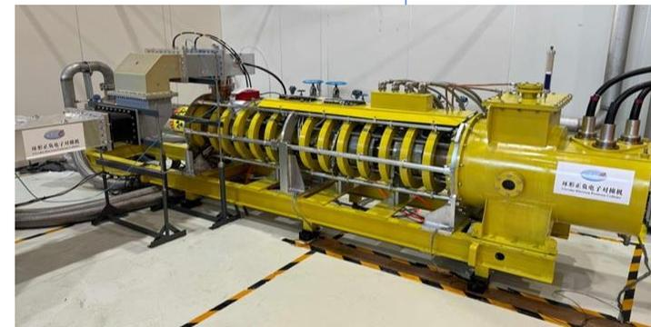
The 2<sup>nd</sup> Klystron (tested)
