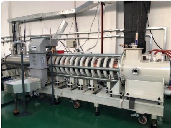
The 1<sup>st</sup> Klystron (tested)
