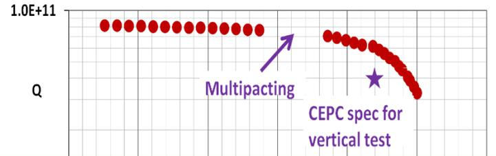
Vertical test of 650MHz 1-cell Cavity
