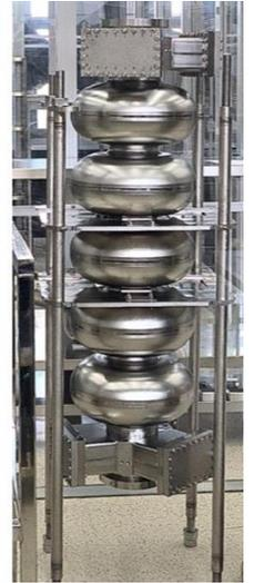
Vertical test of 650 MHz 2-cell cavity
