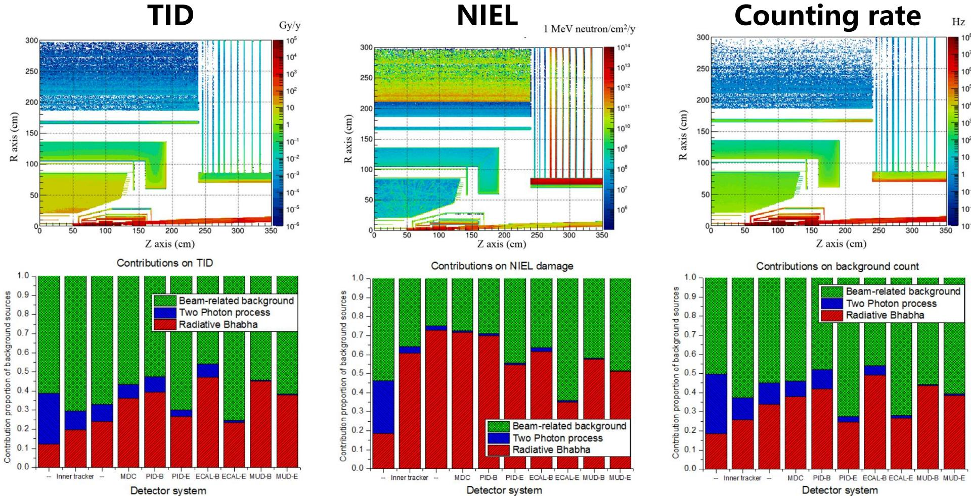
**Inner most detector layer:**  $\sim 3.5 \text{ kGy/y}$ ,  $\sim 2 \times 10^{11} \text{ 1MeV n-eq/cm}^2/\text{y}$ ,  $\sim 1 \text{ MHz/cm}^2$
