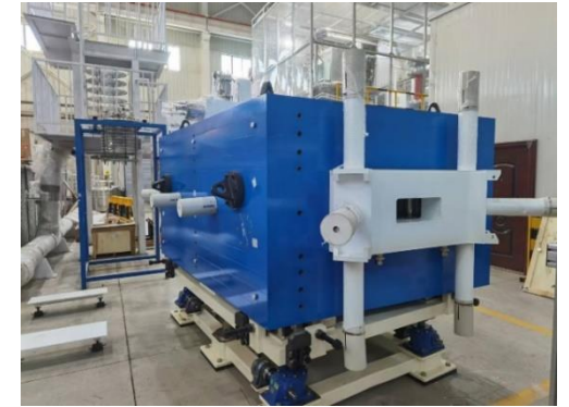
Superferric bending magnet with warm iron
