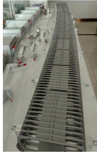
The arc chambers for bending magnet of BRing
