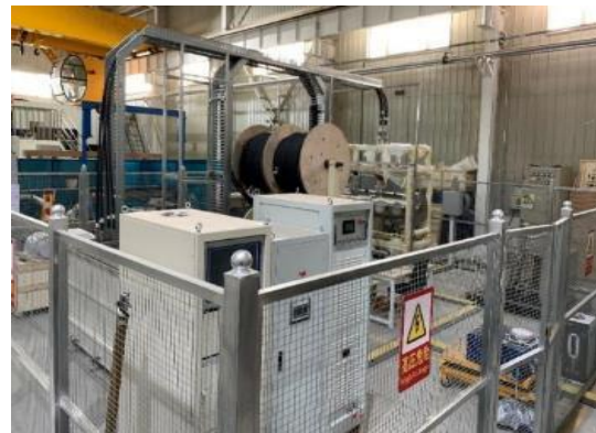
Kicker power supply test with real load
