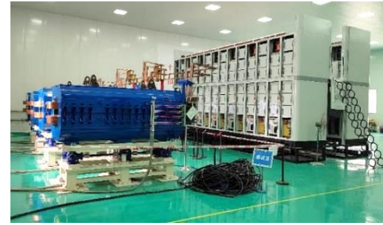
Field measurement of bending magnets
