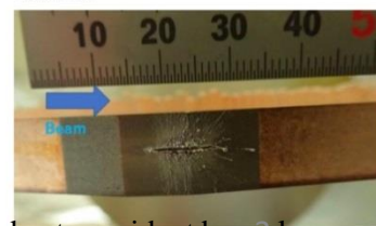
Fig.2 Damage to collimator jaw due to accident beam loss in the SuperKEKB
