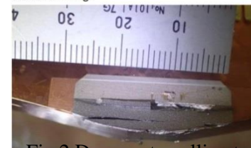
Fig.2 Damage to collimator jaw due to accident beam loss in the SuperKEKB
