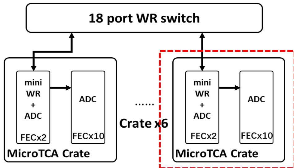
Clock synchronization system structure
