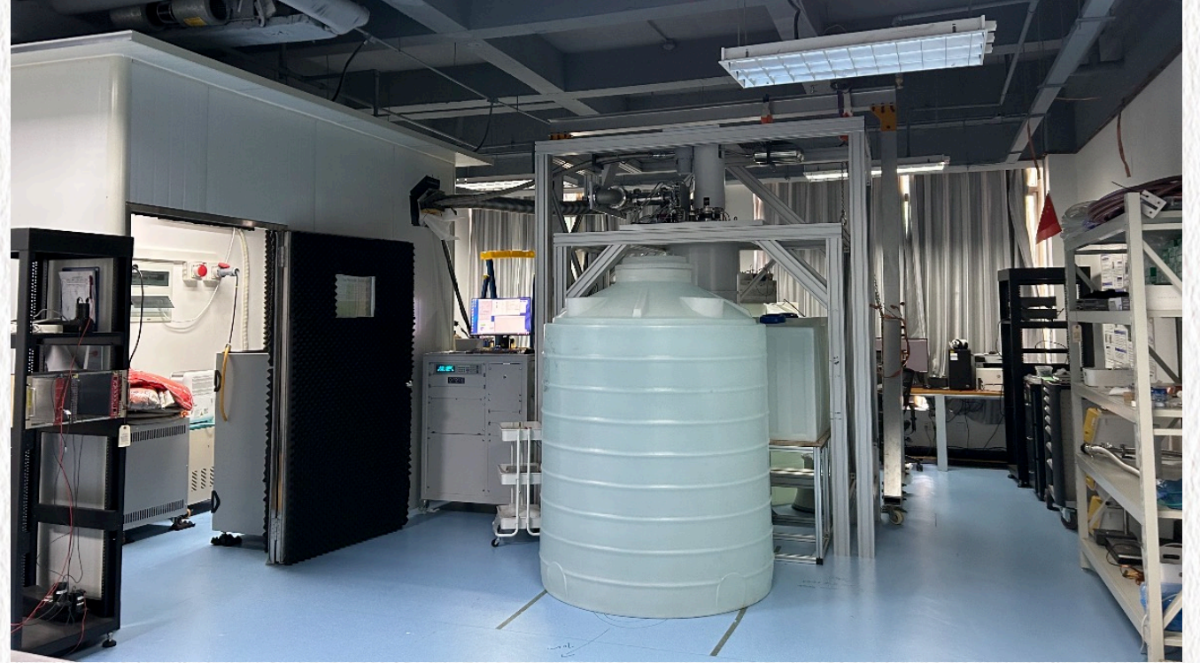
Running with water shielding, reduce pile-up
