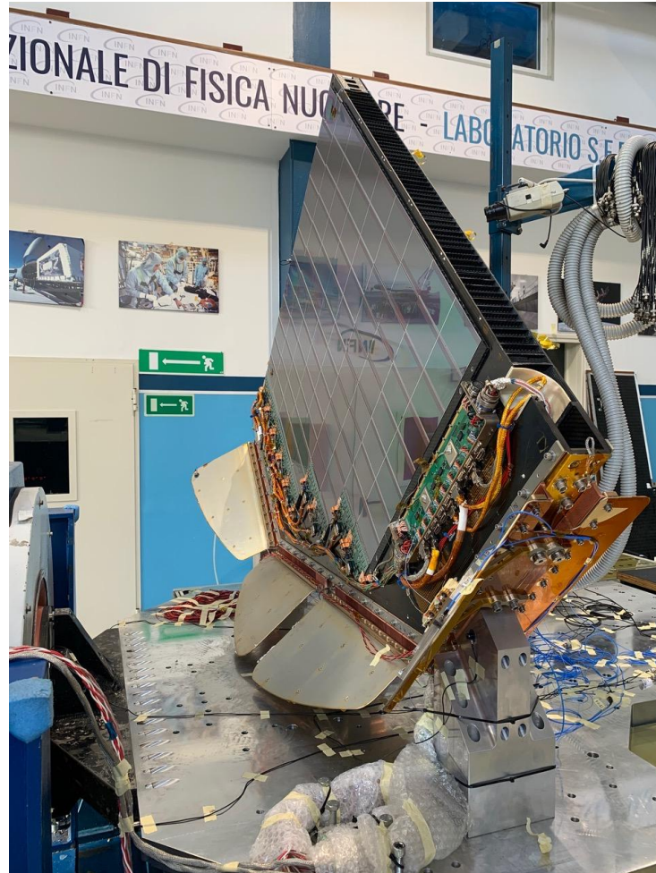
vibration test: no bonding-wire failure
