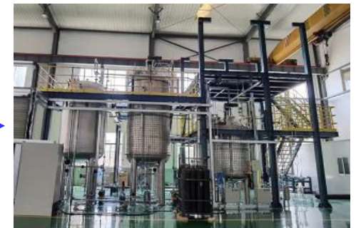
Mixing LAB with PPO and bis-MSB
