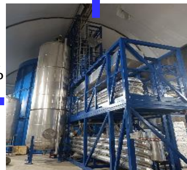
4) Gas stripping to remove Rn and O 2
