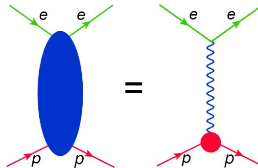
Two methods (both based on one-photon exchange) to study proton form factors
