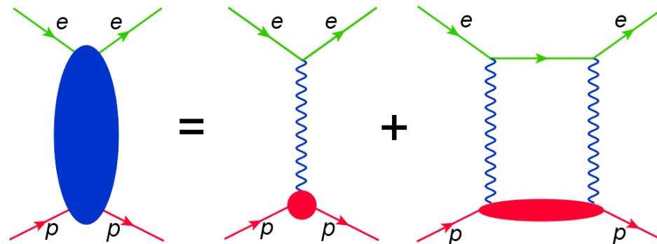
Two methods (both based on one-photon exchange) to study proton form factors
